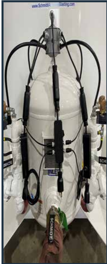
Bulk Blast Pot equipped with the ShortStop PnP
