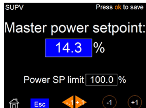
Fig. 6-21 Direct heating power set point page (activated)
